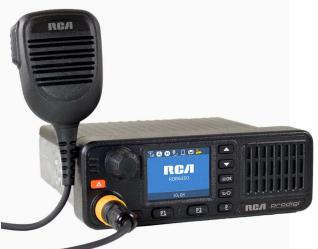
40 Watts, 1024 Channels, Analog, DMR Tier II, III, Prodigi Plus™
